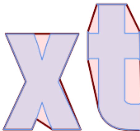
Outer hull simplification of a MultiPolygon, with segmentization
