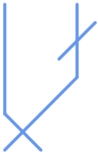
Connected and overlapping linestrings
