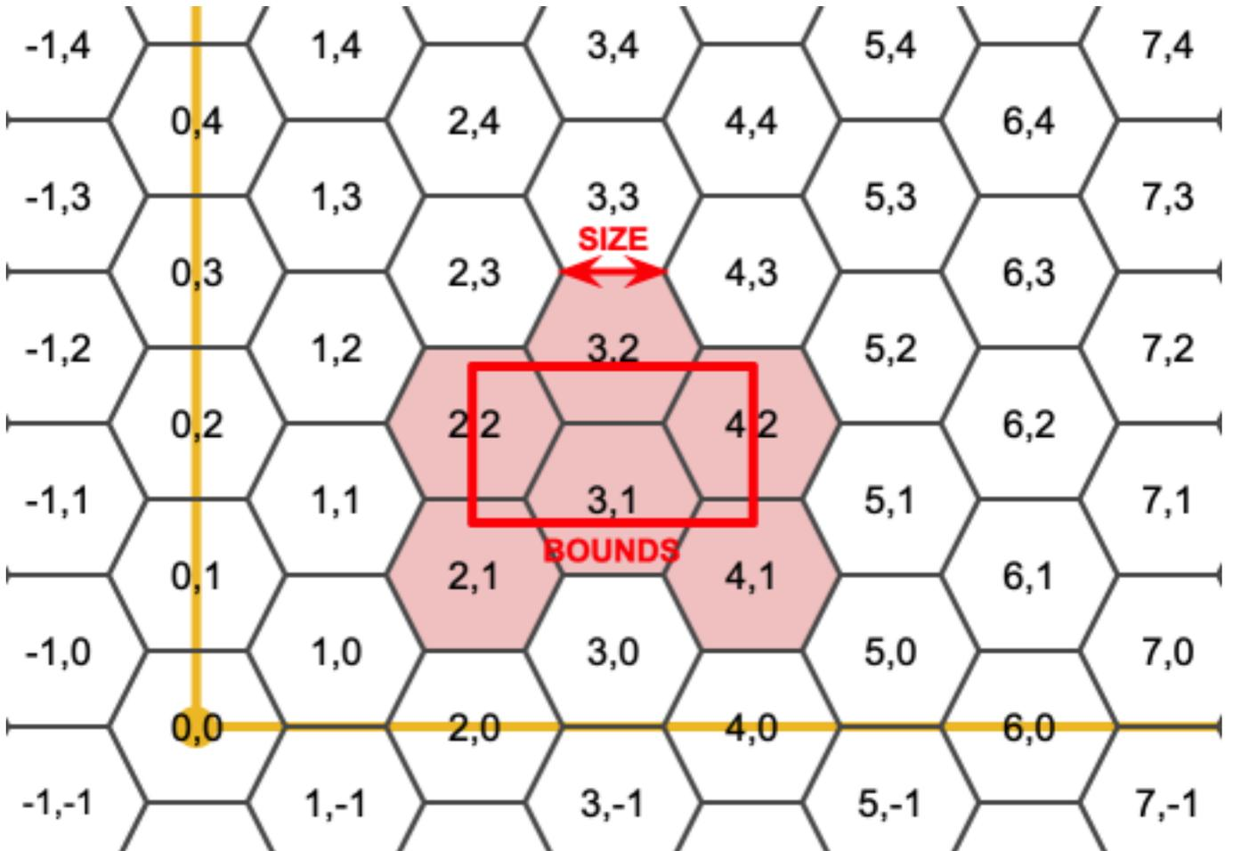
The SRS for the output hexagons is the SRS provided by the bounds geometry.
