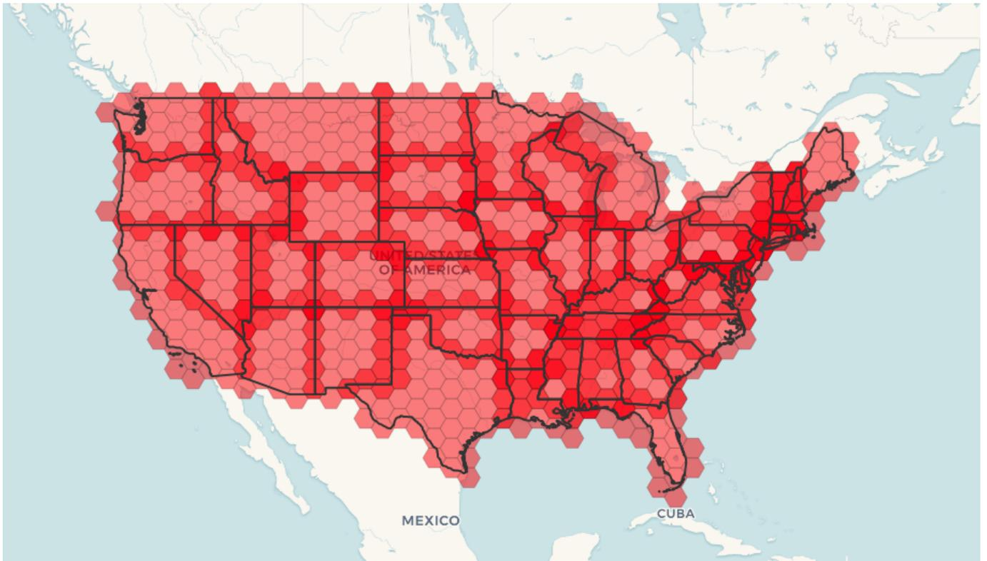
Tiling states results in a hexagon coverage of each state, and multiple hexagons overlapping at the borders between states.
