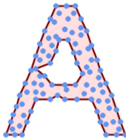
Concave Hull of a MultiPoint, allowing holes (same example as ST_ConcaveHull)
