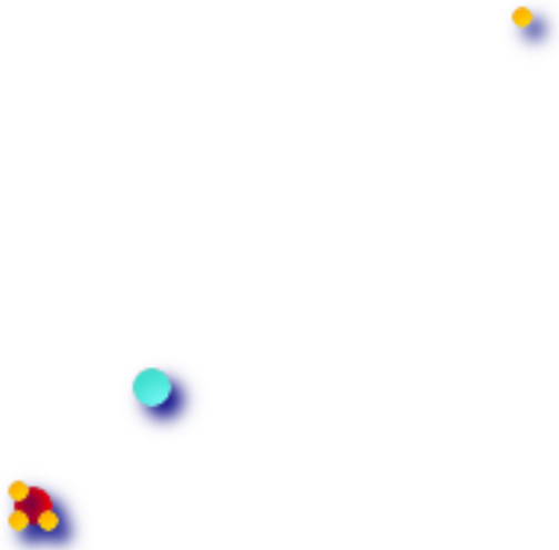
Comparison of the centroid (turquoise point) and geometric median (red point) of a four-point MultiPoint (yellow points).
